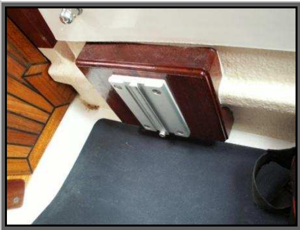
Above the cabin mount with table stowed. The stop screw mentioned in the narrative can clearly be seen
