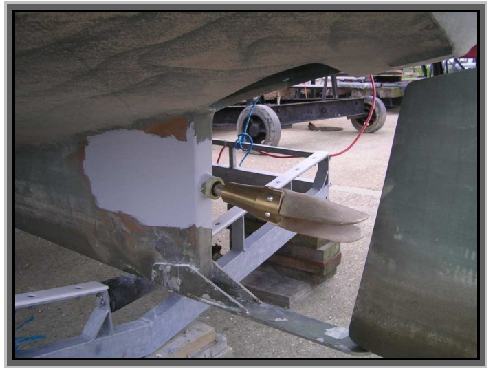
Above: Folding propeller in "sailing" position . Note how it is shadowed by the skeg and its position relative to the rudder blade.
