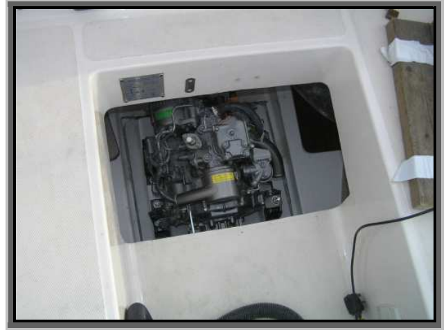
Above: Engine installation looking from the cockpit. David is going to produce a hatch moulding for access which is going to have minimal interference to the cockpit.
