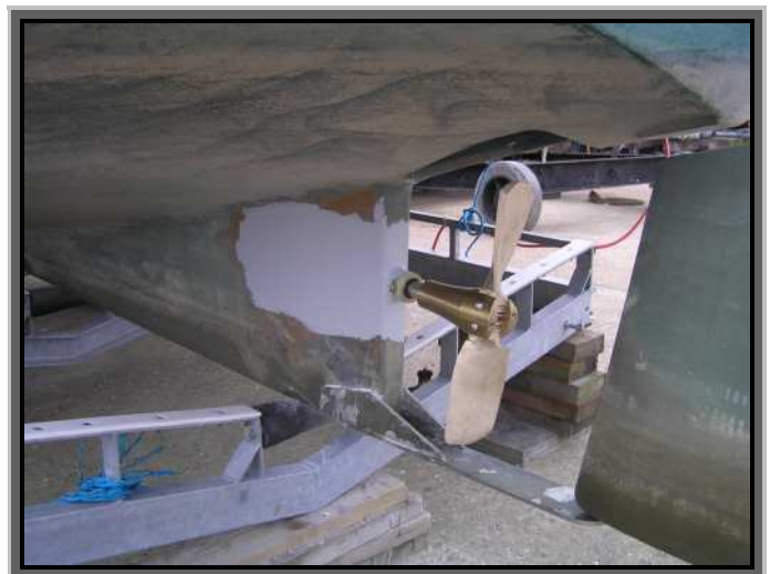
Above: The next trial was made with a folding two blade prop. This will improve sailing performance, i.e reduce drag
